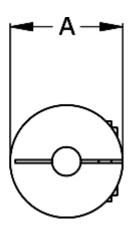
A = 56 D1 = 25 D2 = 30 L = 73 Nom. torque NM (Tkn) = 30
